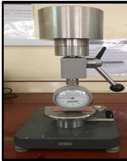
Figure (4) : Shore D hardness tester for cold cure acrylic specimens
