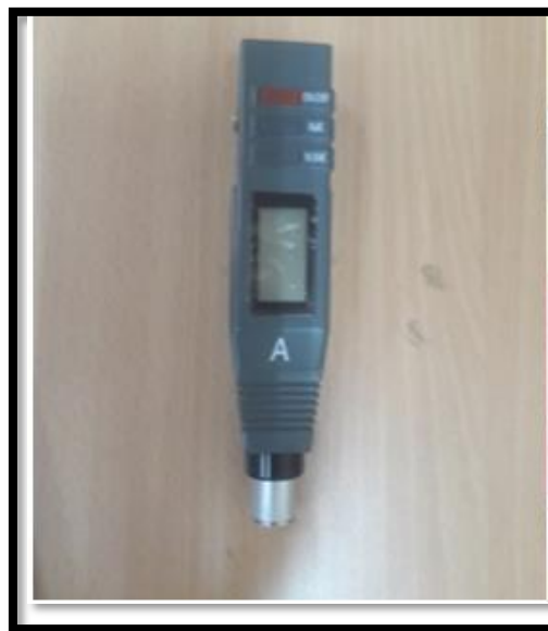
Figure(5): Shore A hardness tester for flexible acrylic specimens
