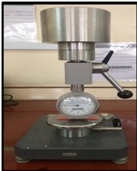
Figure 4: Shore D hardness tester for cold cure acrylic specimens
