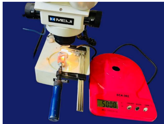
Figure (5): Stereo-zoom microscope with specimen holding device that was particularly constructed to maintain a constant pressure of (5N)
