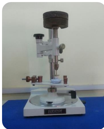
(Figure 3) Five-Kg load applied on each crown during setting time of the cement
