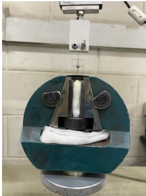
Figure 1: bracket- archwire test unit on Instron machine.
