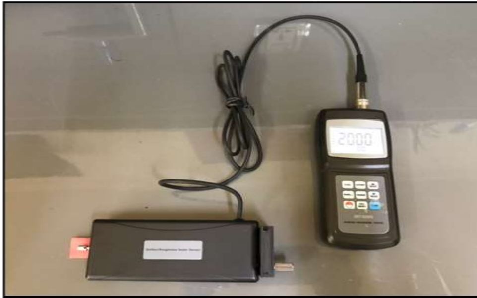
Figure (1): Specimen under the profilometer device for surface roughness test
