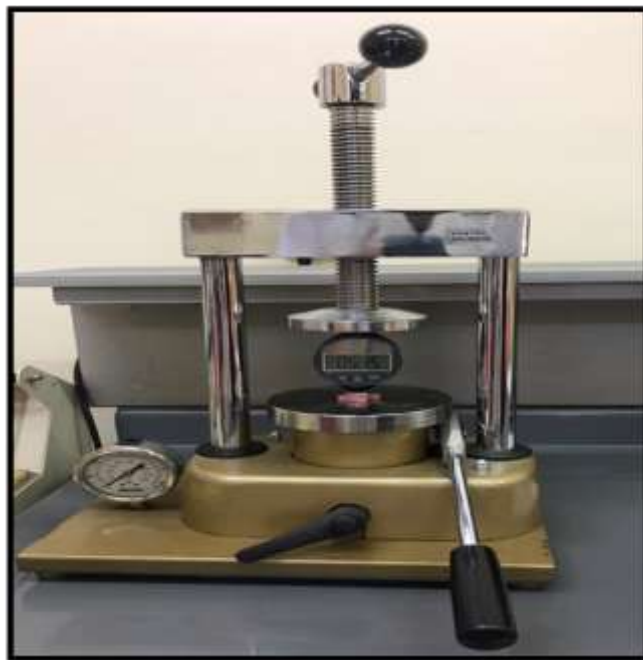
Figure (2): specimen under the Shore D device for surface hardness test
