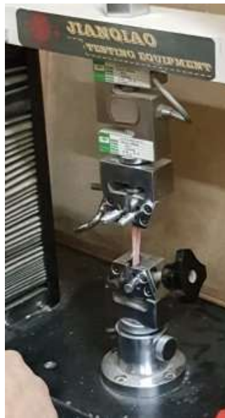
Figure 2. The specimen tested for the tensile strength in Instron testing machine
