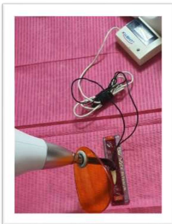
Figure 1 light curing of composite resin and place of thermocouple
