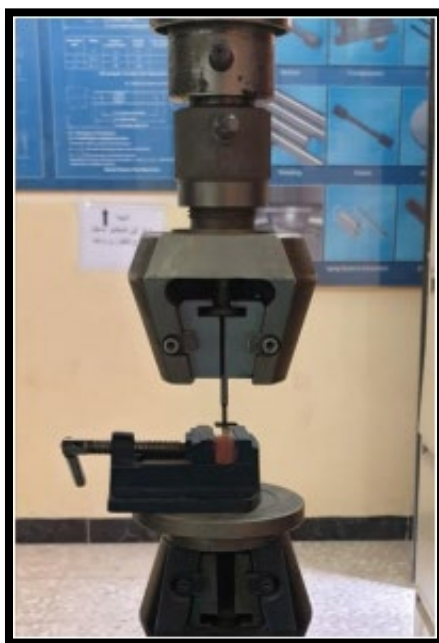
Figure 3: The computer-controlled universal testing machine used in the study (Rod application used for axial compression test).
