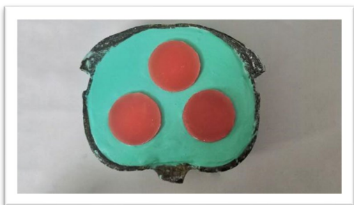
Figure 4: wax pattern for the stone mold.
