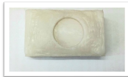
Figure 3: Silicone mold for the wax pattern fabrication.
