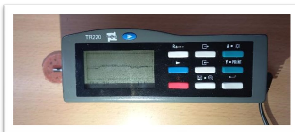
Figure 8: Soft liner specimen under surface roughness test
