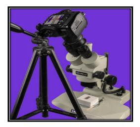
Figure (3): Imaging the resin blocks with standardized position of stereomicroscope and digital camera.
