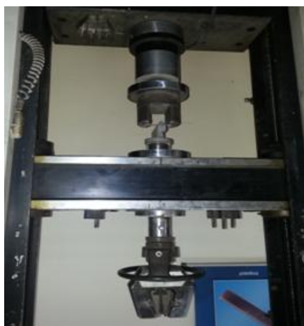
Figure 2. Specimen under transverse strength test
