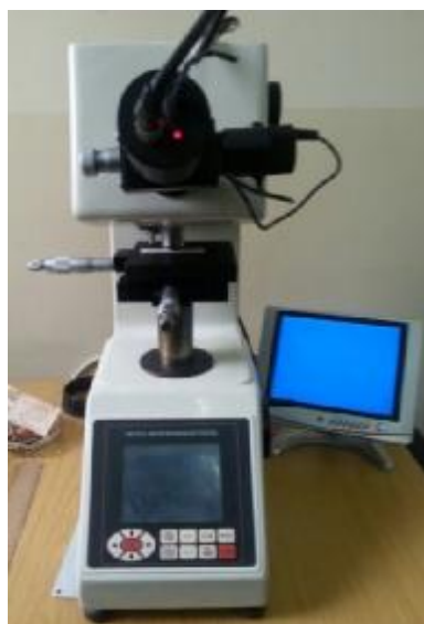
Figure 3. Specimen under hardness test
