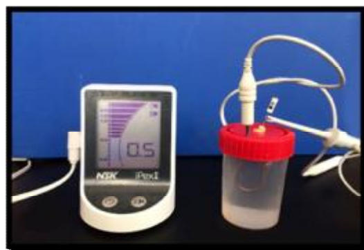
Figure (4): Experimental model and iPex II electronic apex locator.
