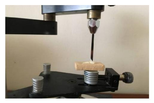
Figure (1) Bracket bonding procedure with the help of a surveyor for applying a constant force
