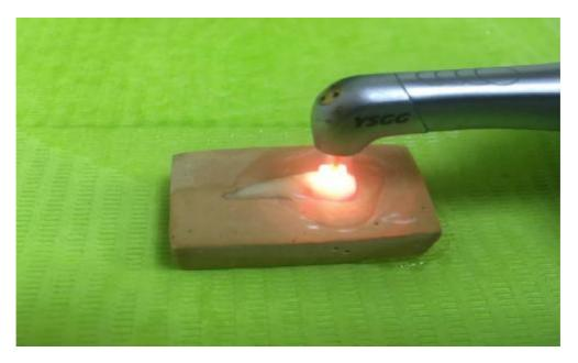
Figure (2) bracket debonding using water atomized laser
