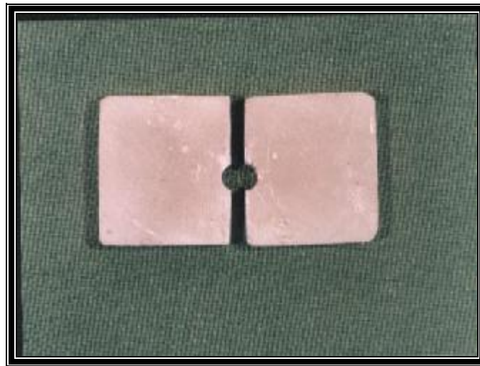
Figure 1: An aluminum mold of 8-mm in height and 4-mm in diameter was used as a mold for the composite material for measuring the depth of cure.
