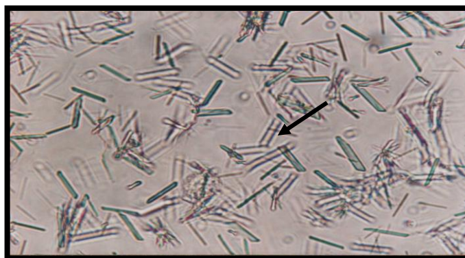
Figure 1: The calcium sulphate dihydrate crystals for the control group at different time intervals
