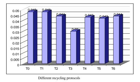
Figure 2: Bar-chart for the mean load deflection of Ni-Ti arch wire after different recycling protocols
