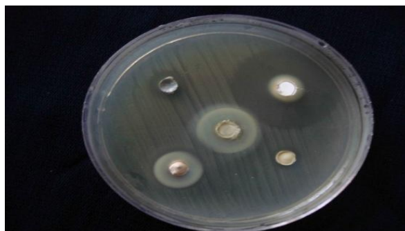
Fig. 6 Agar diffusion method of Endodontic sealer on Enterococcus faecalis on Mueller Hinton Agar media
