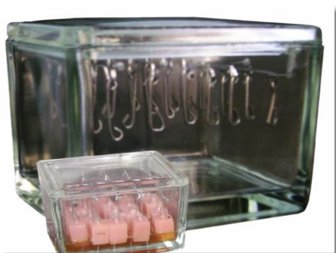
Figure 3: Glass trough and teeth attached to the suspenders (20 suspenders receiving 20 sample).
