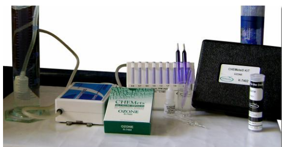
Figure 2: Ozone generating device with tubing and stone and the ozone CHEMets®Kit.
