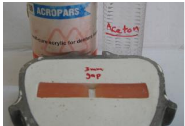
Figure (6) Combination of [Acetone and monomer] wetting with fine brush (No. zero)
