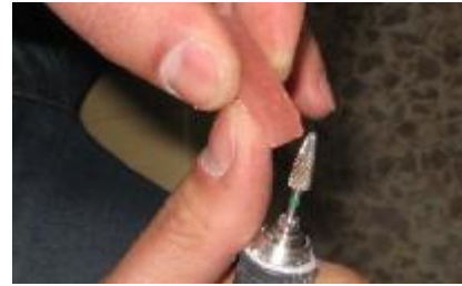
Figure (3 b) the cut end was prepared with acrylic bur with 45 degree bevel
