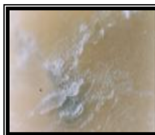
Fig. (16): Cohesive failure (X4).
