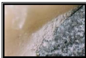
Fig. (17): Mixed failure (X4).
