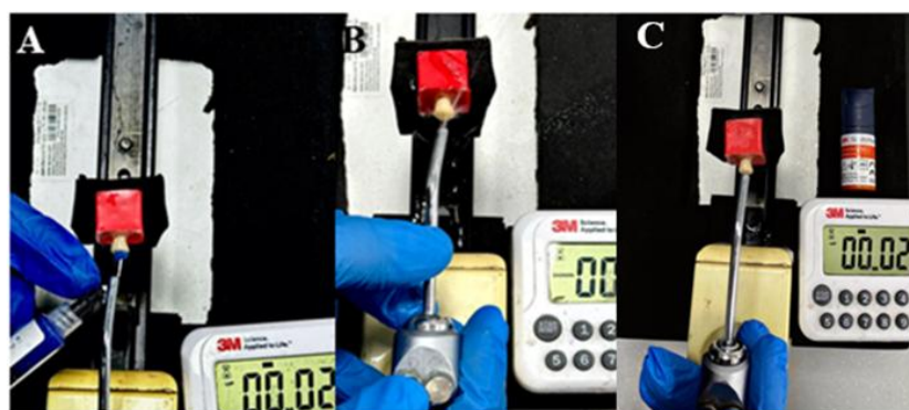
Figure 3. A: dentin etching for 3sec. B: rinsing dentin for 15 sec. C: air drying for dentin
