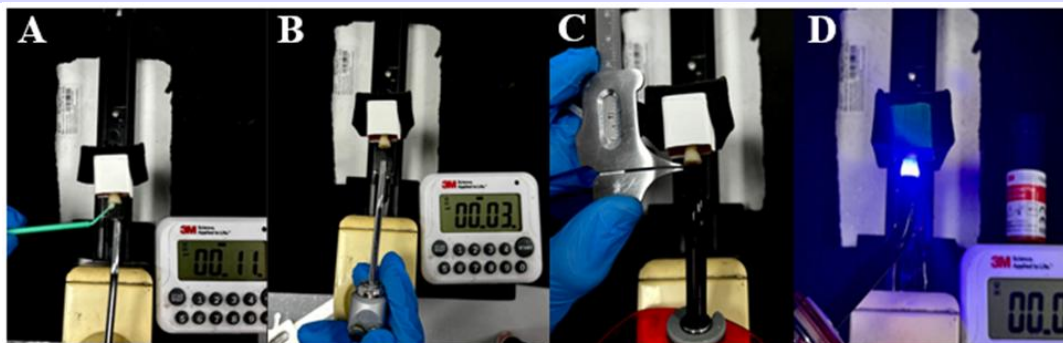
Figure 2. A: Bonding application with micro brush B: Air drying C: measuring 1mm distance from dentin surface D: light cured for 20 sec.
