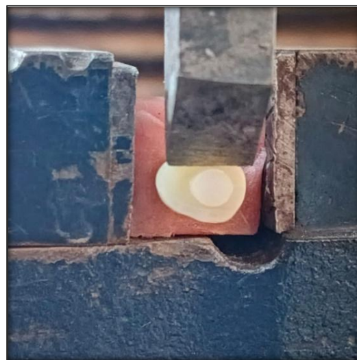
Figure 9. Universal testing machine sample in lower jaw of machine.
