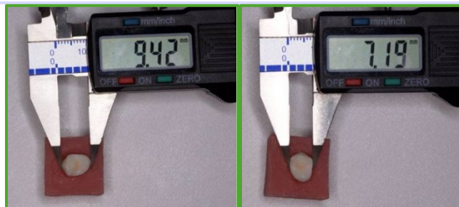
Figure 1: Measuring BP and MD dimensions by a digital caliper.
