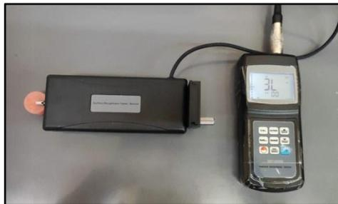
**Fig 3:** Roughness tester
