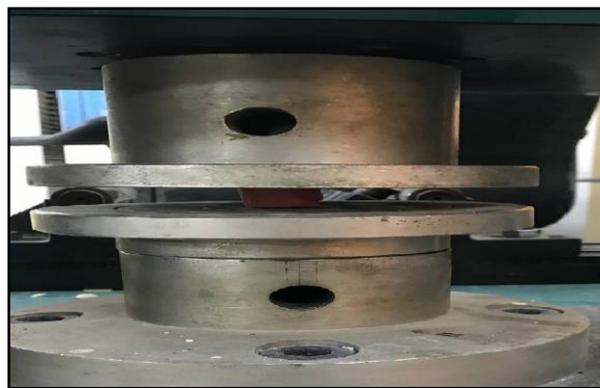
**Fig 2:** Sample under compressive strength device
