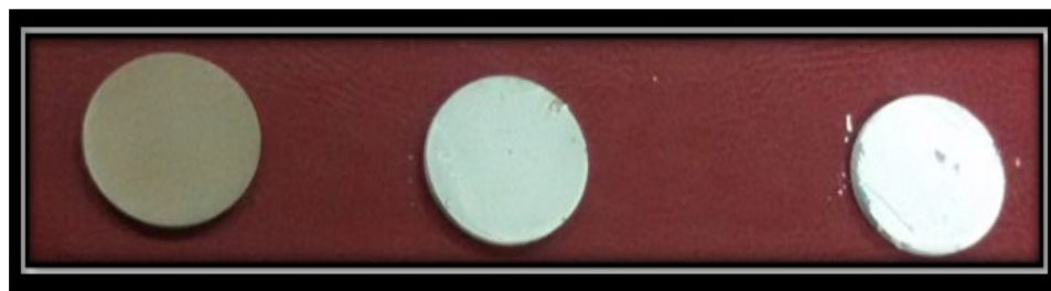
Figure 1: CP Ti discs (a) Uncoated, (b) nano HA coating, (c) mixture of nano HA &TiO 2 nano HA coating
