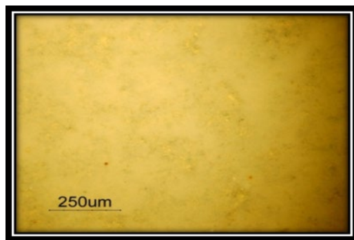
Figure 6: Optical micrographic Nano HA coated disc surface with no cracks in the coating layer
