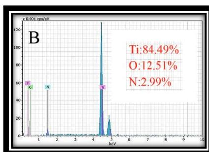
**Figure 4:** EDS of titanium substrate textured by CO<sub>2</sub> laser.
