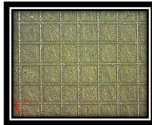
**Figure 2:** Optical microscope pictures X40 of CO<sub>2</sub> laser pattern.
