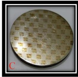
**Figure 1:** Topographic images: CO<sub>2</sub> textured titanium discs.
