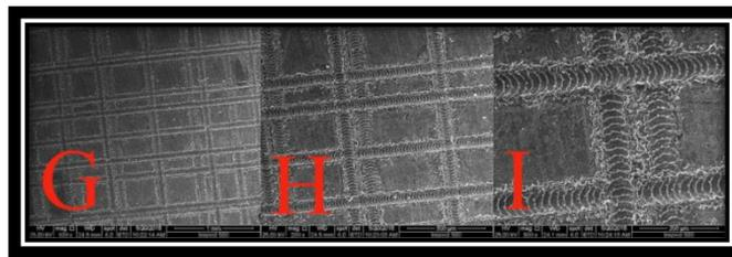
**Figure 3:** SEM micrographs of titanium surfaces textured using a CO<sub>2</sub> laser.
