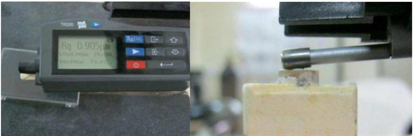
**Figure 1.** Profilometer measuring the surface roughness of a specimen.
