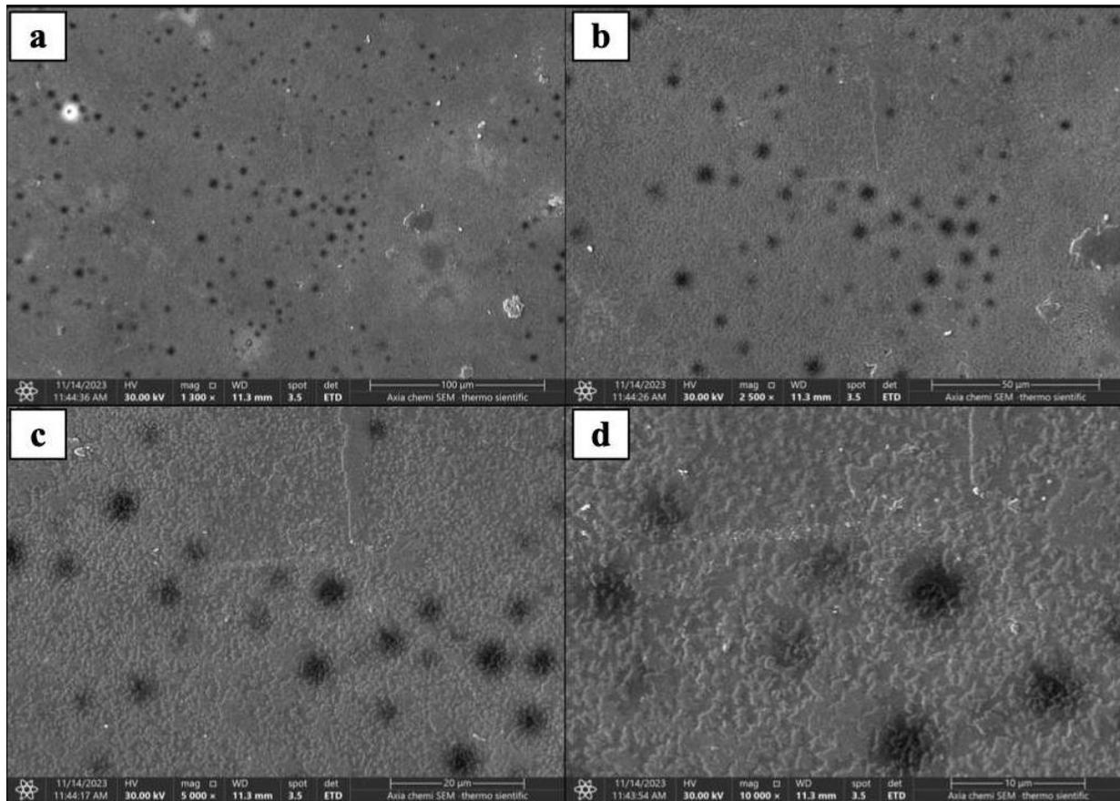
**Figure 3.** SEM for Group A zirconia specimen (Un-treated zirconia) at a) 1300x magnification, b) 2500x magnification, c) 5000x magnification, d) 10000x magnification.
