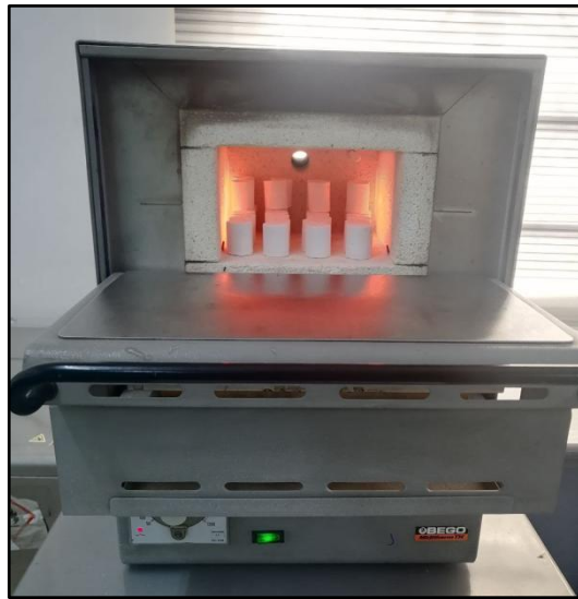
Figure 1: Investment specimens heated using model drying oven
