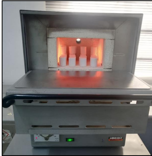
Figure 1: Investment specimens heated using model drying oven
