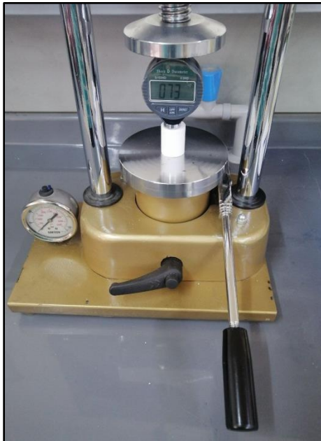
Figure 2: Investment specimen under surface hardness Shore D durometer unit
