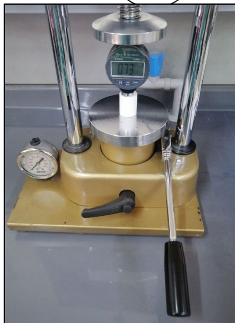
Figure 2: Investment specimen under surface hardness Sore D durometer unit
