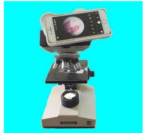
Figure (6): LabCam microscope adapter
