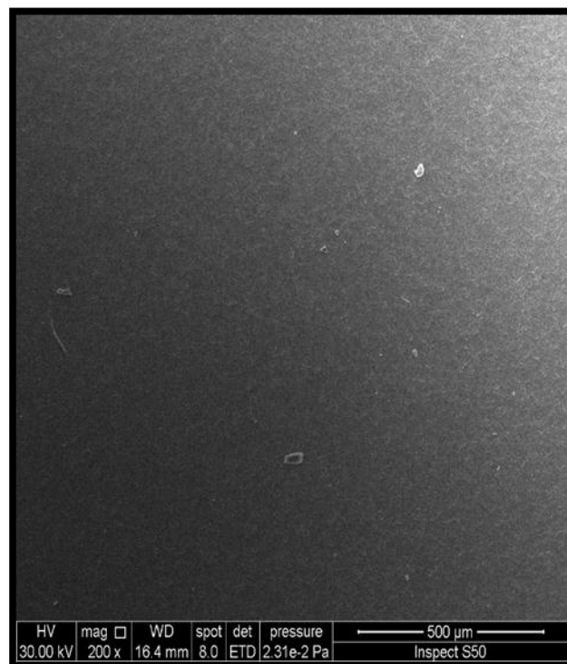
Figure (4-D): SEM for zirconia specimens treated with a combination of 50μm of aluminum-oxide and 5% of hydrofluoric acid .
