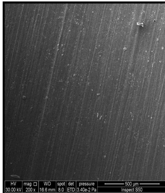
Figure (4-C): SEM for zirconia specimens treated with 5% of hydrofluoric acid .
