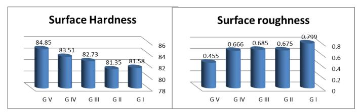
Figure (2): Bar chart showed the surface hardness and surface roughness for all groups.
