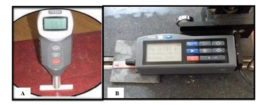
Figure (1): A. Surface hardness test, B.Surface roughness test.
