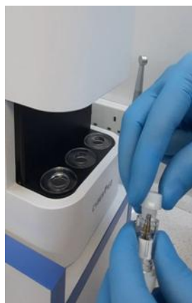
Fig. (5): CORE Plasma activator device for plasma surface treatment
