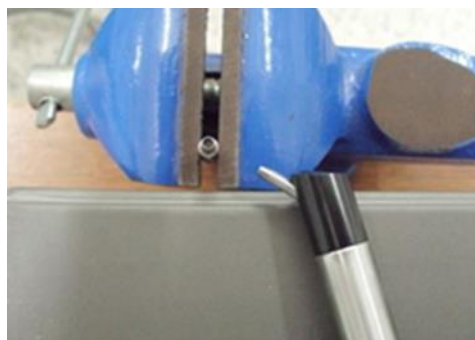
Fig. (4): Sandblast surface treatment for Ti-abutment.
